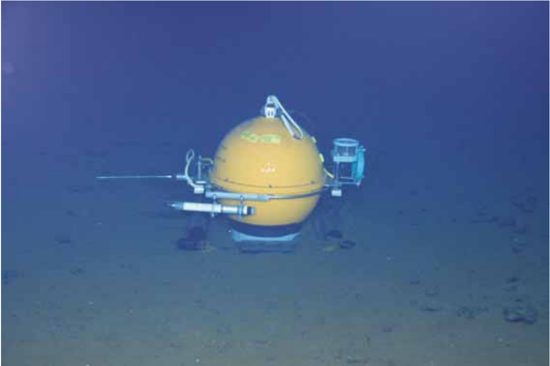
Fig. 2. The BBOBS on the seafloor at the FP6 station, which is 200 km south of the Macdonald hotspot. The depth is 4400 m.
